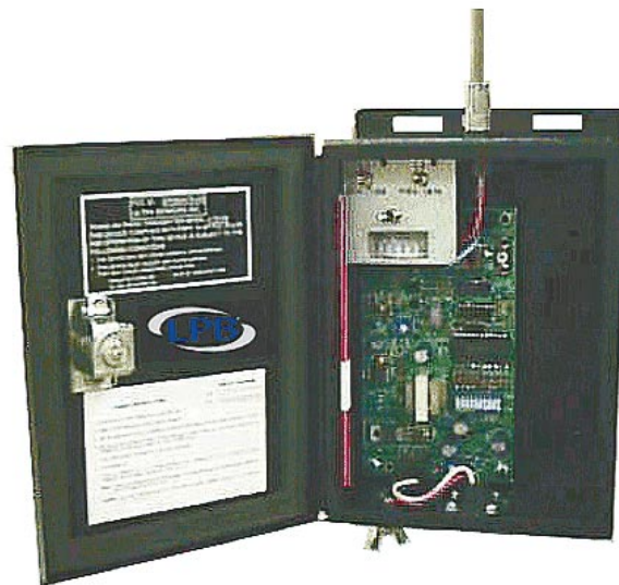
The interior of the LPB AM-2000 transmitter: Tune it up and get on the air
